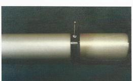
LINE UP THE HOLES IN THE WEBBING AND THE MAST AND RIVET THE WHOLE ASSEMBLY IN PLACE.
